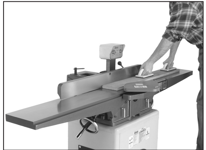
Figure 26. Typical surface planing operation.
